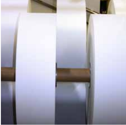
▲ At Spinnaker Coating, rolls are slit at three locations on the company's eight slitters, three of which are 78 in. wide.
