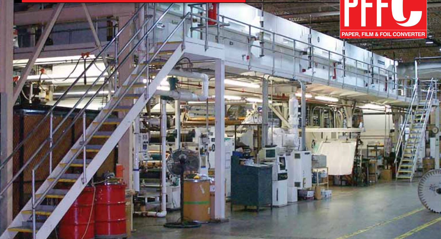
▲ A 60-in. Black Clawson silicone coater operates at 1,400 fpm.
