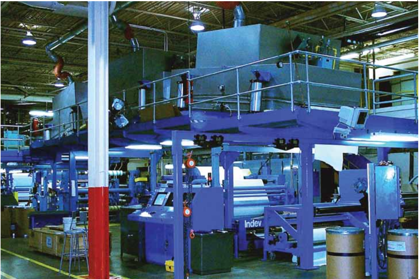
▲ At Spinnaker Coating, rolls are slit at three locations on the company's eight slitters, three of which are 78 in. wide.
